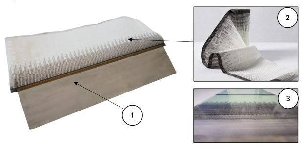
The BF2S2525 connecting element consists of a 3.0 mm thick flat profile 1. Different lengths and widths of the profile are available. Two layers of the hybrid FAUSST fabric are joined to the profile by means of roll seam resistance welding 2. After embedding in the FRP, the component can be joined via the metal profile 3.
